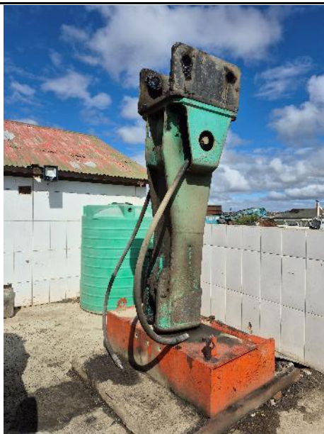
Stand for the hydraulic breaker effectively preventing oil spills
